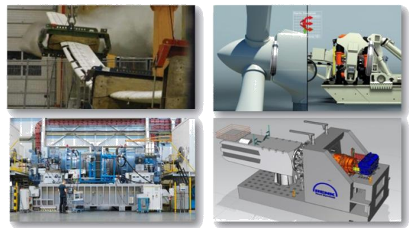
Figure 5: Risø National Laboratory blade test ; FAG bearing test rig ; ZF Wind Power Antwerpen NV gearbox test rig ; 7.5MW drivetrain test rig – Renk test systems
