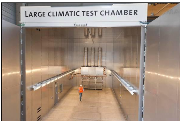
Figure 8: OWI-Lab's large climatic test chamber
