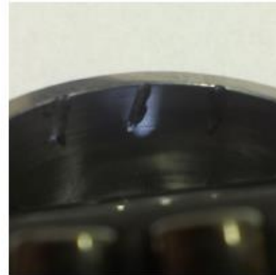
(c) Three small, shallow grooves to imitate an outer-raceway fault.
