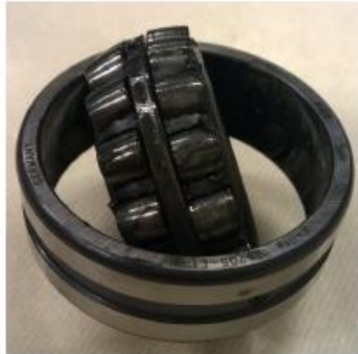
(a) Mildly inadequately lubricated bearing outside the housing.
