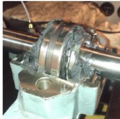
(b) Healthy Bearing in an open housing.
