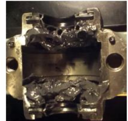
(d) Grease reservoir in the bottom of the housing.
