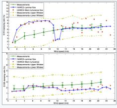
igure 5 : Damping ratios of the first Fore-Aft (top) and Side-Side (bottom) modes versus vind speed for a turbine in operation
