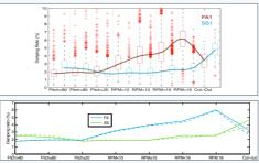
Figure 4 : Damping overview for the first Fore-Aft (FA) and Side-Side (SS) modes for (top) 2012 with box plots to indicate the spread. (bottom) Results for 2012 (full) and 2013 (dashed) are consistent. The x-axis represents different operational conditions or states of the offshore wind turbine
