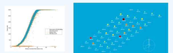
Figure 11: Estimated power curve vs warranty power curve (left) Wind farm overview of power curve deviation for a given wind sector (right)
