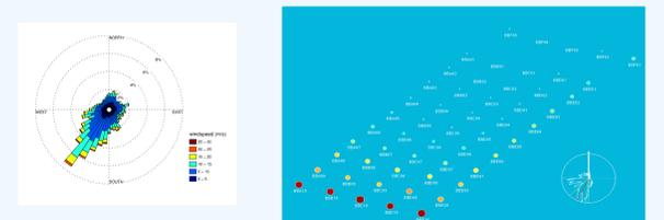
Figure 10: Wind Rose (left) Wind farm overview showing averaged produced power and wake losses for a given wind sector
