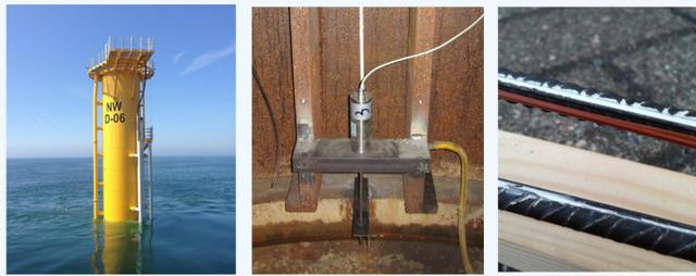
Figure 3: Picture of a transition piece in the Northwind wind farm (left) Installed displacement sensor (middle) optical fiber Bragg sensor embedded in a steel bar (right)
