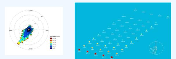
Figure 10: Wind Rose (left) Wind farm overview showing averaged produced power and wake losses for a given wind sector (right)
