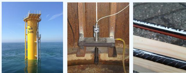
Figure 3: Picture of a transition piece in the Northwind wind farm (left) Installed displacement sensor (middle) optical fiber Bragg sensor embedded in a steel bar (right)
