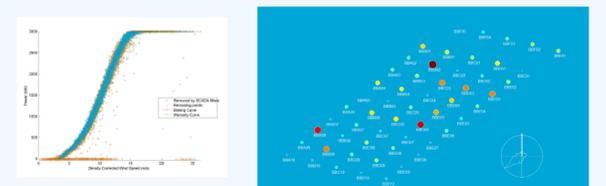
Figure 11: Estimated power curve vs warranty power curve (left) Wind farm overview of power curve deviation for a given wind sector
