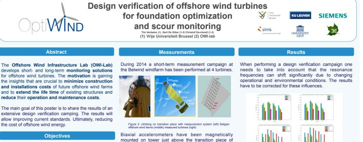
In design verification the resonance frequencies of the fundamental tower modes are identified using a mobile measurement system and state-of the art operational modal analysis techniques. The obtained frequencies are compared with the as designed values
