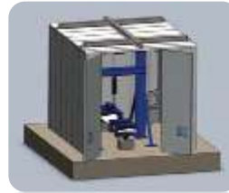
Load & climate testing blade materials
