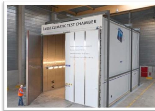
Wind turbine component Test Lab with large climate chamber (Temperature testing)
