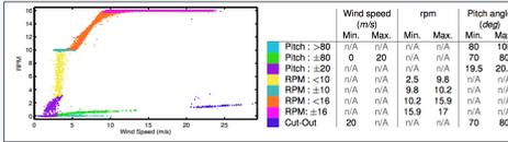
Figure 3: (left) RPM vs. wind speed with colors indicating the different operational cases (right) Definitions of the different operational cases
