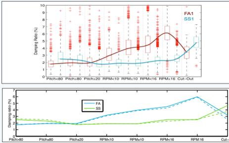
Figure 4 : Damping overview for the first Fore-Aft (FA) and Side-Side (SS) modes for the top 2012 with box plots to indicate the spread. (bottom) Results for 2012 (full) and 2013 (dashed) are consistent. The x-axis represents different operational conditions or states of the offshore wind turbine
