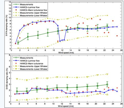
Figure 5 : Damping ratios of the first Fore-Aft (top) and Side-Side (bottom) modes versus wind speed for a turbine in operation
