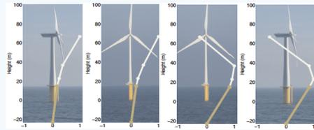
Figure 1: Fundamental tower/foundation modes in parked conditions. From left to right: first for-aft mode, first side-side mode, second side-side mode, second for-aft mode
