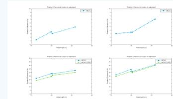
Figure 9: Relative difference between measured frequencies and as designed values versus waterdepth
