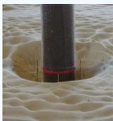
Scour holes have a significant effect on the resonance frequencies. **With increasing scour depth the resonance frequency will decrease.** This can potentially induce resonant behavior.
