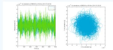
Figure 4: Example measured vibrations in for-aft and side-side direction (left) topview of motion (right)
