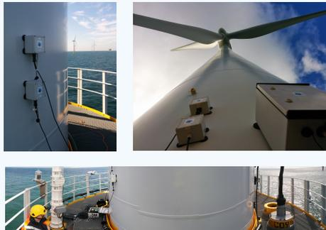
Figure 3: magnetically mounted accelerometers and data acquisition system (top) panorama picture during measurements (bottom)
