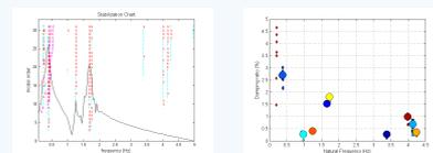
Figure 6: automated operational modal analysis: stabilization diagram (left) frequency damping cluster plot (right)
