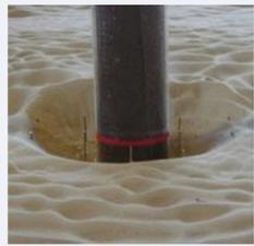
Figure 1: Example of scour near a monopile foundation
